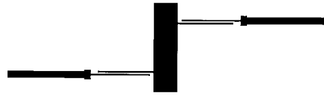
Fig. 6. Layout of the microstrip filter with the central resonator connected at the voltage minima for the full-wavelength resonance (width of input line: 0.56 mm, coupling length: 4.5 mm, length of first resonator: 5.19 mm, length of second resonator: 4.88 mm, width of central resonator: 2.06 mm, length of central resonator: 7.75 mm, remaining data as with Fig. 3).
